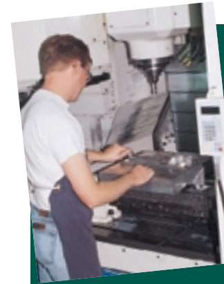
Son Jason Baker, the night shift lead, sets up the shop's newest Okuma machining center, an MA-550VB vertical with high-speed spindle.
